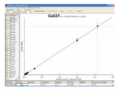
The carbon curve (right) demonstrates a very good fit with low alloy steels and carbon steels.
